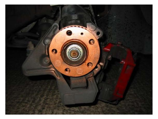
8. Put the new disk in place and put in the retaining screw
