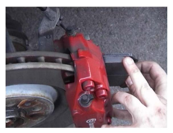
18.Slide the bottom of the two stainless pins in from the back to the front (reverse of before) as picture below. The pin goes in the back hole of the calliper, through both holes in the pads and through the front hole in the calliper. If you can't push it through all the way with your hands use the drive punch and a little tap with the hammer
