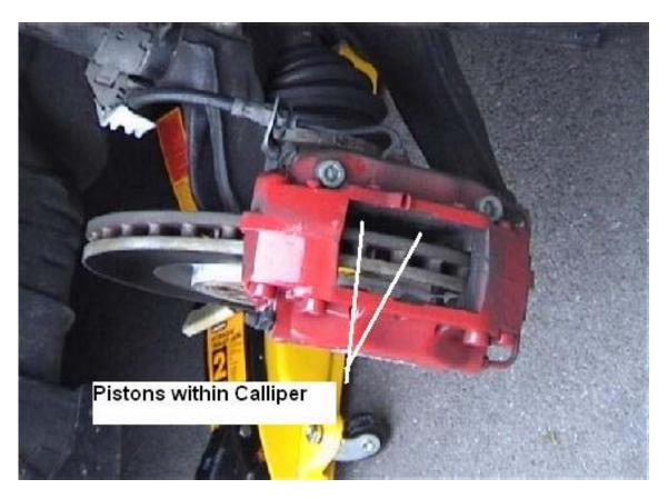
16. Apply copper grease to the back of the pad ONLY, do one at a time and put plenty on. I didn't put quite enough on in the picture below and they squeak so a bit more than this.
