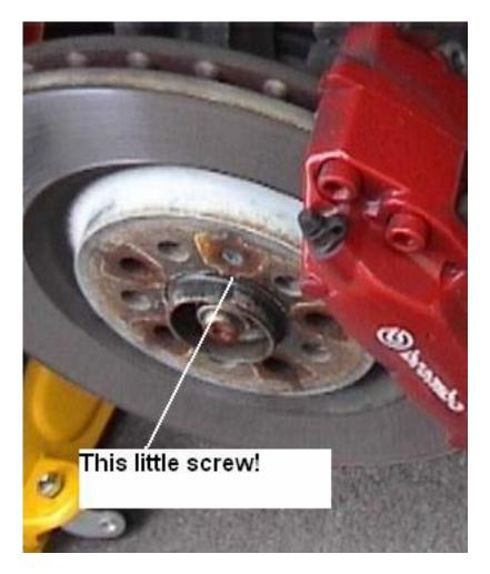
6. While you have the disk off you may want to clean up the area, use a wire brush if necessary and then wipe down with a cloth to remove the bits of brake dust and any rust etc.
